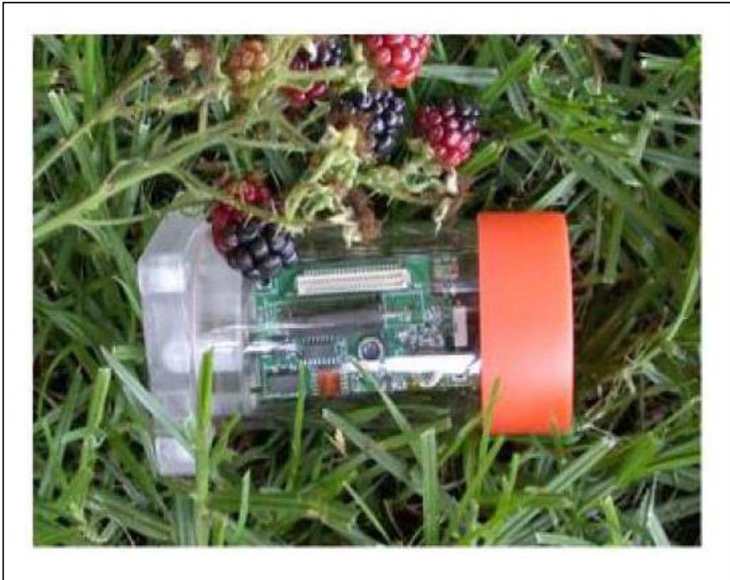
Figure 5 Deployed sensor nodes with acrylic enclosure [10]
