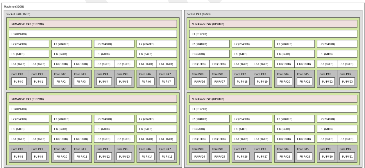
Figure 4 Memory hierarchy of AMD bulldozer.
