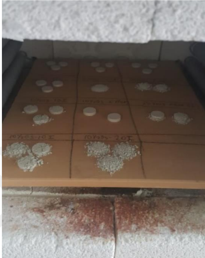
Figure 64: Samples containing semolina dispersed after the burn out process.
