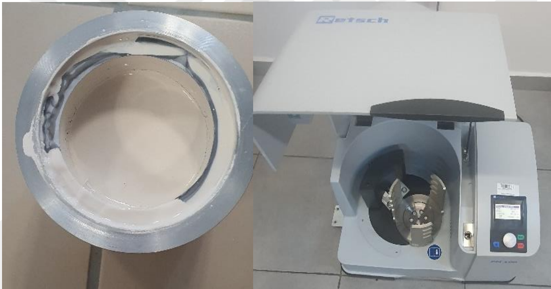
Figure 44: Planetary ball milling device and the \text{Si}_3\text{N}_4 jar with slurry inside.
