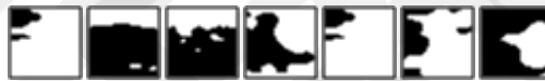
Figure 32: 32x32 frame results in a bearing with shoe trail defects on outer diameter.
