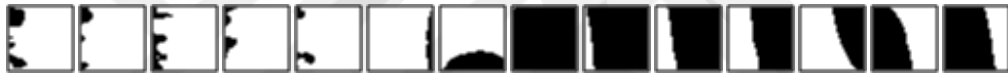
Figure 38: 32x32 frame results in a bearing with impact defects on outer diameter.
