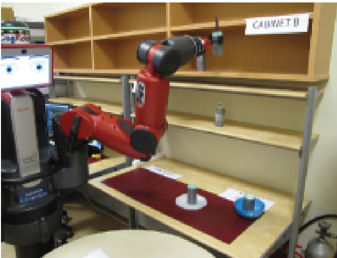
Figure 2. The robot is picking up an object from Cabinet B and placing it on kitchen table.
