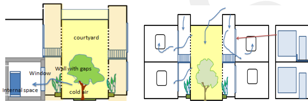
Figure 4.26: Cooling Solutions; the cold air enters the interior space through gaps on walls then the glass windows, which located behind the walls
