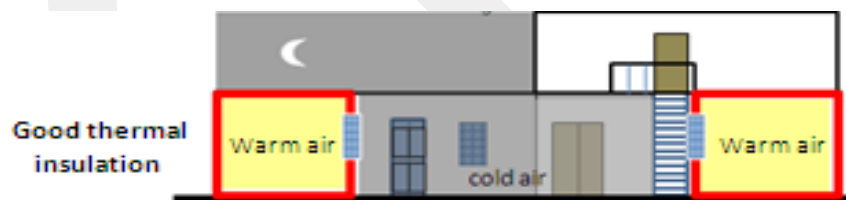
Figure 3.51: Heating system 3; in the winter at night, cold air collects in the courtyard and the good isolation of the walls helps to isolate the internal space from the external space.
