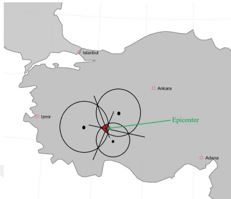
Figure 1.1: A process called triangulation uses seismic data from three locations to identify the epicenter of an earthquake.
