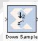
Figure 48: Xilinx System Generator - Down Sample Block Symbol
