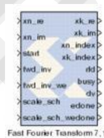
Figure 61: Xilinx System Generator - Fast Fourier Transform 7.1 Block Symbol
