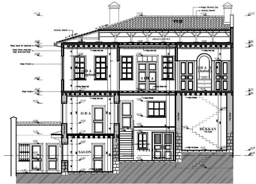
Figure 147. Registered buildings / B-B Section: 1/50
