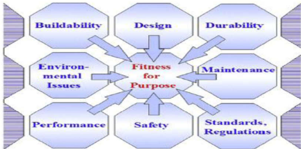
Figure 2.6: Parameters for PV Building Integration[43]
