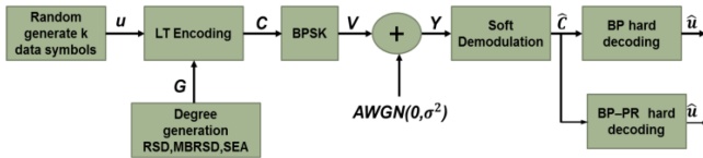
Figure 2. System model for soft-demodulation-hard-decoding approach.
