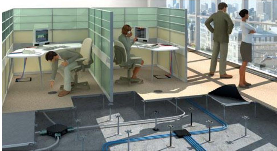
Figure 17: Raised flooring systems
