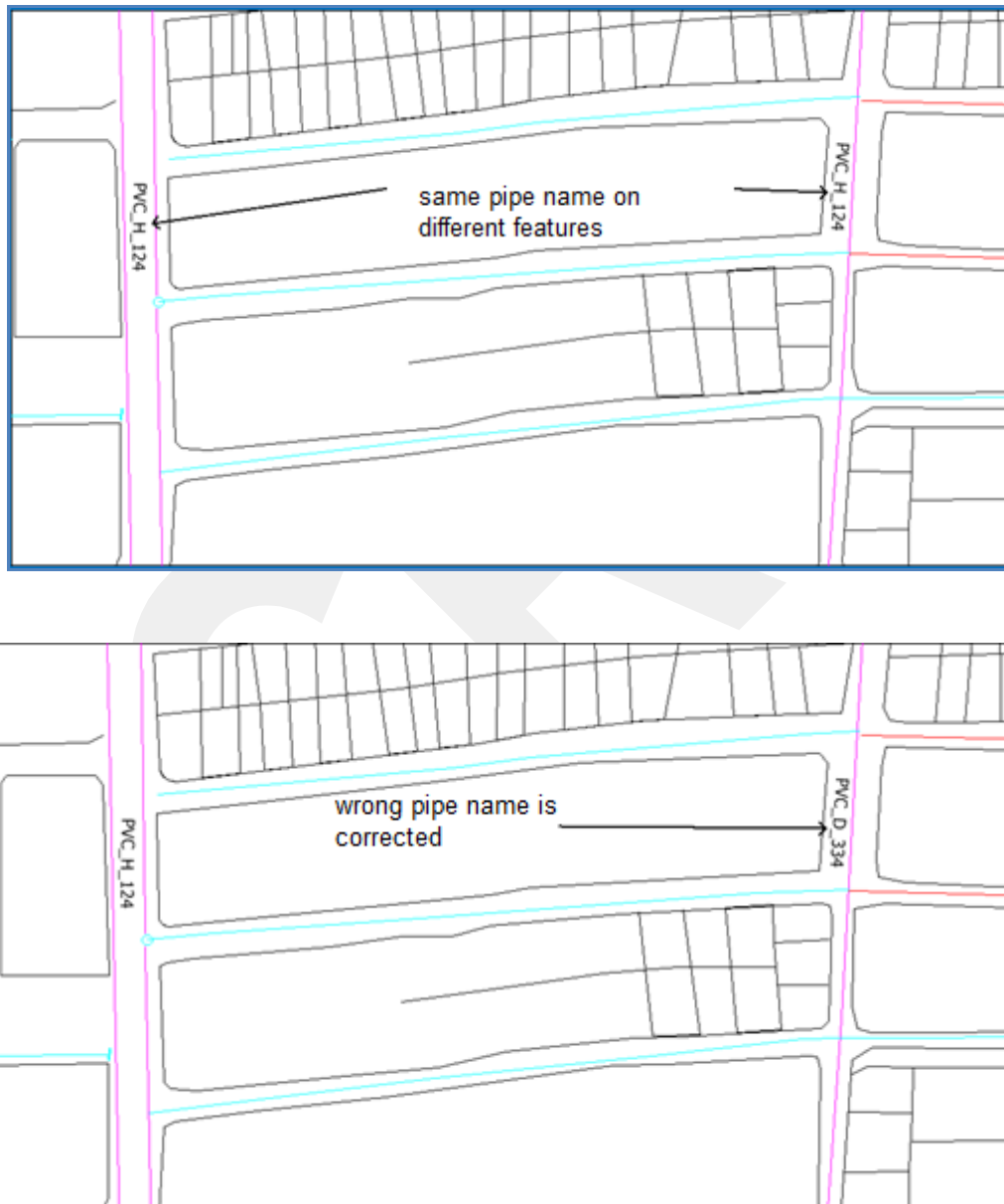
Figure 4.10 Wrong pipe names
