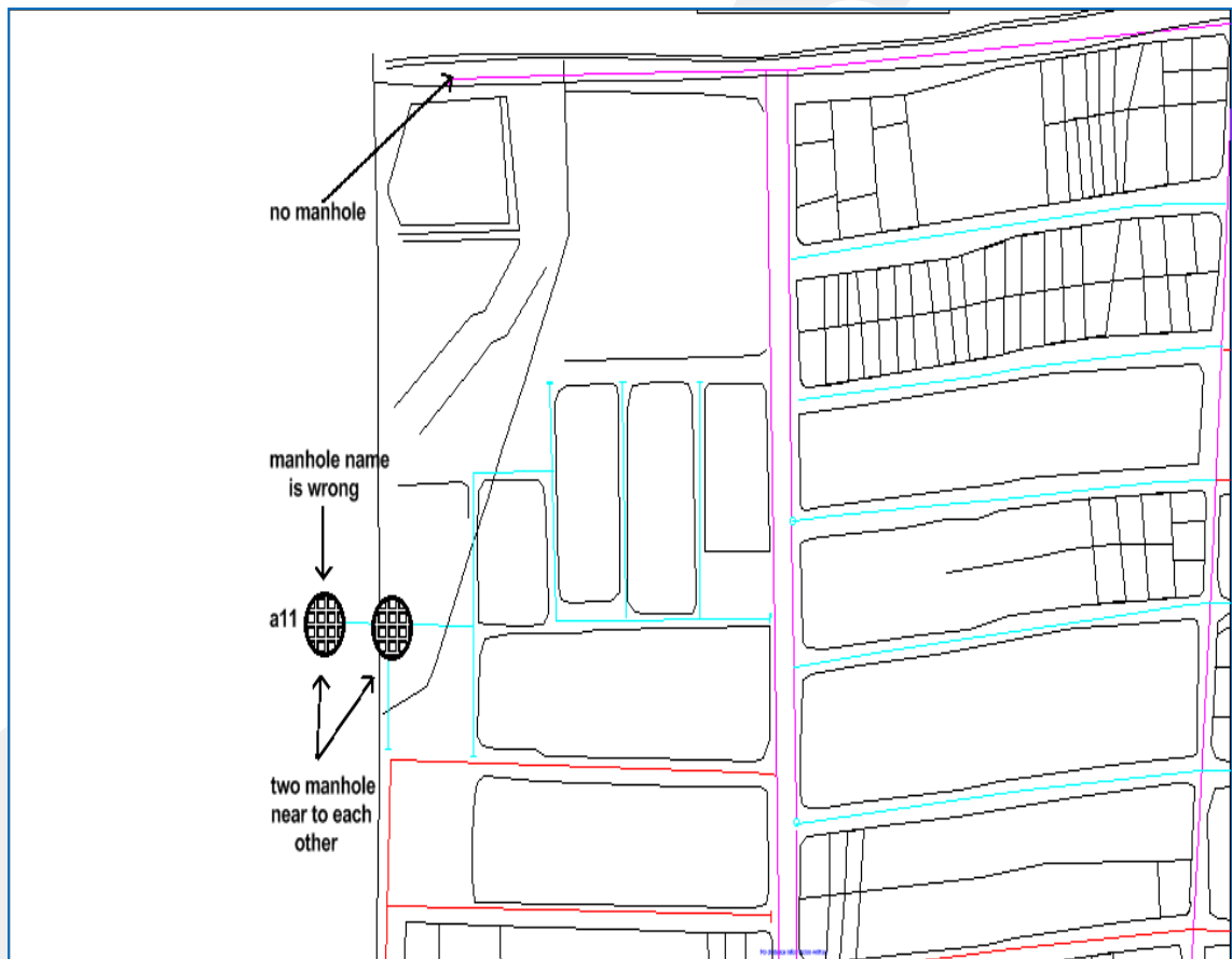
Figure 4.14 Two manholes are too close to each other.
