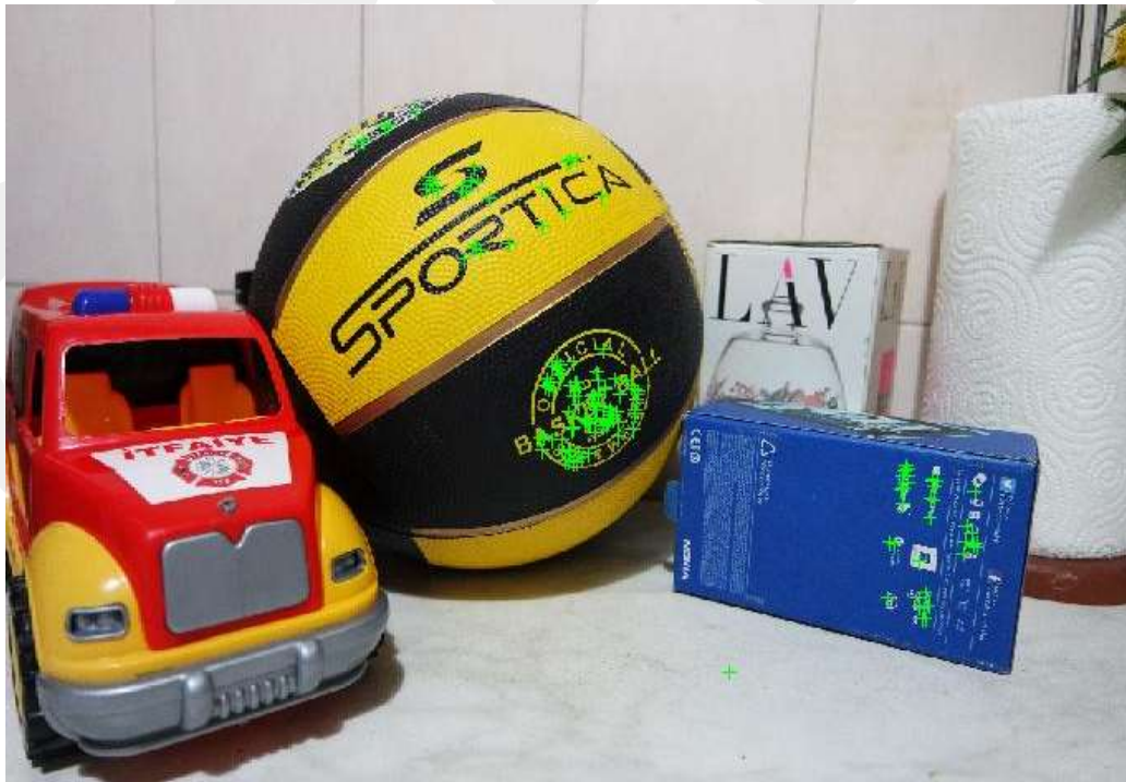
Figure 6.20: The Strongest corners from the first image (second test)
