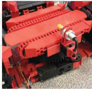
Figure 41: Rotary table component
