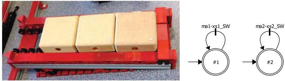
Figure 32: Exit Slide component and its models G_{XS1}, G_{XS2}
