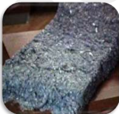
Fig 5.2. Cotton Batt Insulation (Hussein, 2012, p.6).
