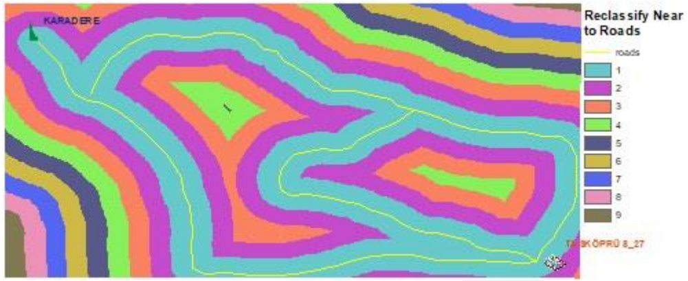
Figure 59 Reclassified raster layer for near to roads for the extent between Karadere Dam and Taşköprü Substation
