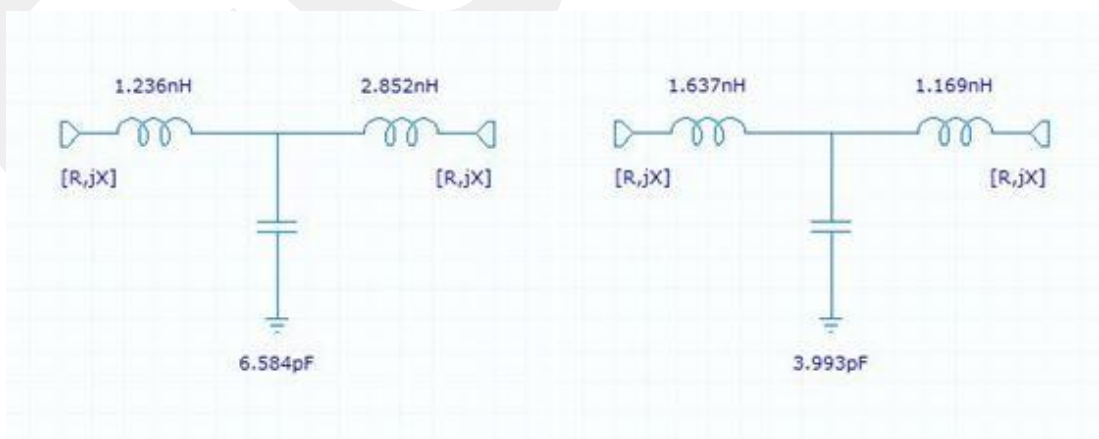
Figure 23 Input and output impedance matching circuits (left -input matching, right -output matching)
