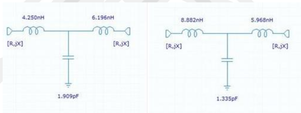
Figure 6 Input and output matching networks (left-input, right-output)
