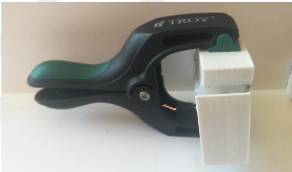
Figure 3.8: Test Specimen Placed and Clamped On Bending Test Setup from Different Angle of View.
