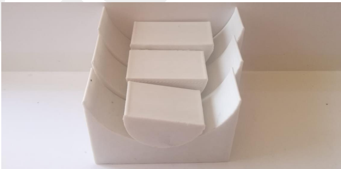
Figure 3.1: Width Comparison of Bending Test Setup Apparatus.
