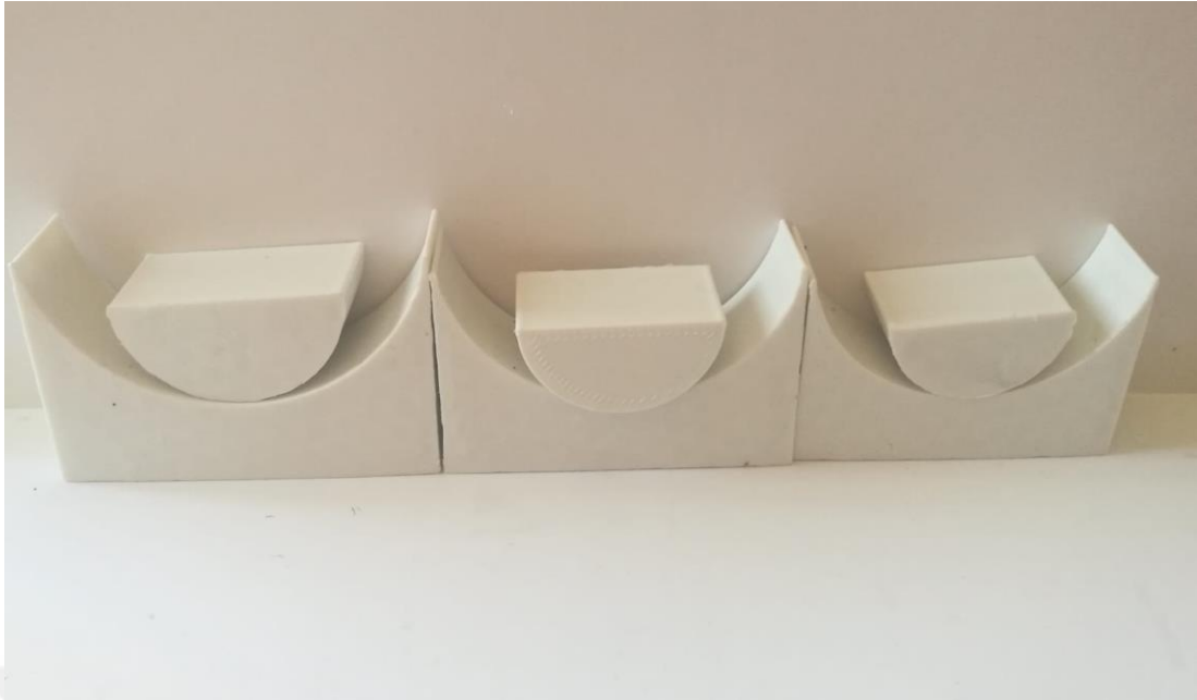
Figure 3.2: Height Comparison of Bending Test Setup Apparatus.
