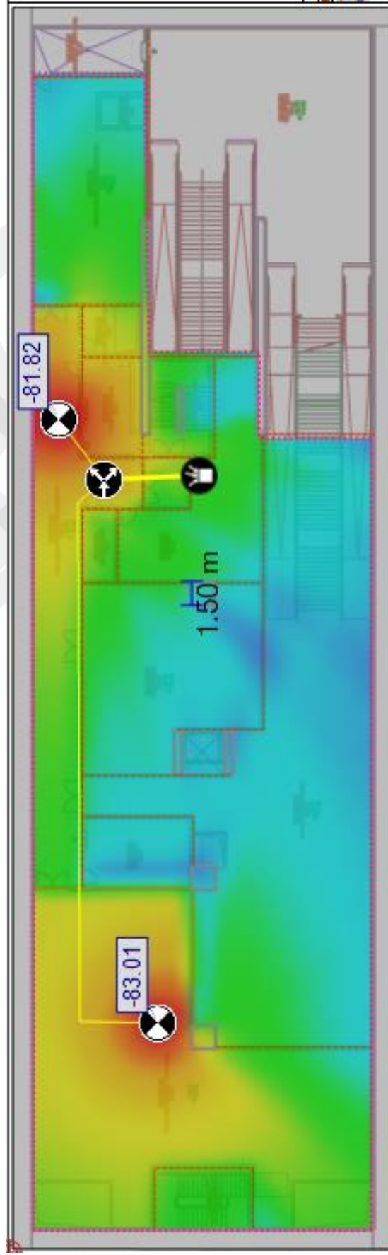
Figure 39: 2D Simulation result with a metal plate/reflector on the side two walls
