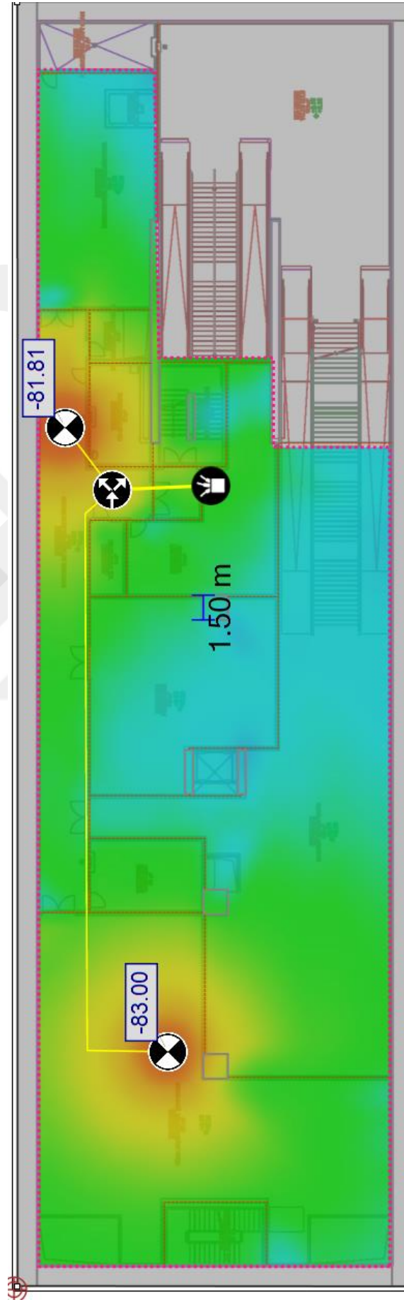
Figure 33: Antenna transmissions at technical volume
